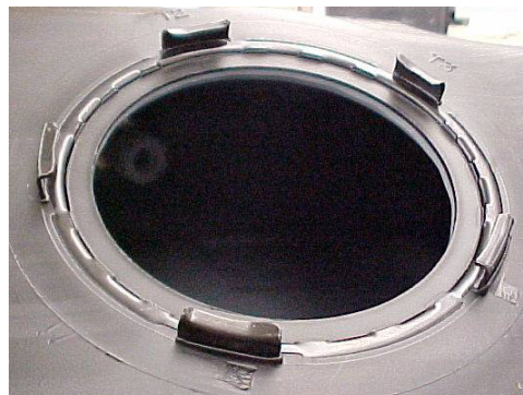
Figure E: Flat sealing surface
